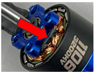
The red arrow points to the Star center connection wiring endpoint that is covered with shrink tubing and tucked between the mounting bracket and stator wiring.
